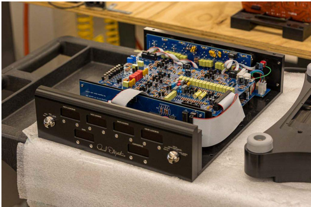
A closer look at the “phono stage” of the Momento series. In essence, this is four phono pres in a common enclosure.
