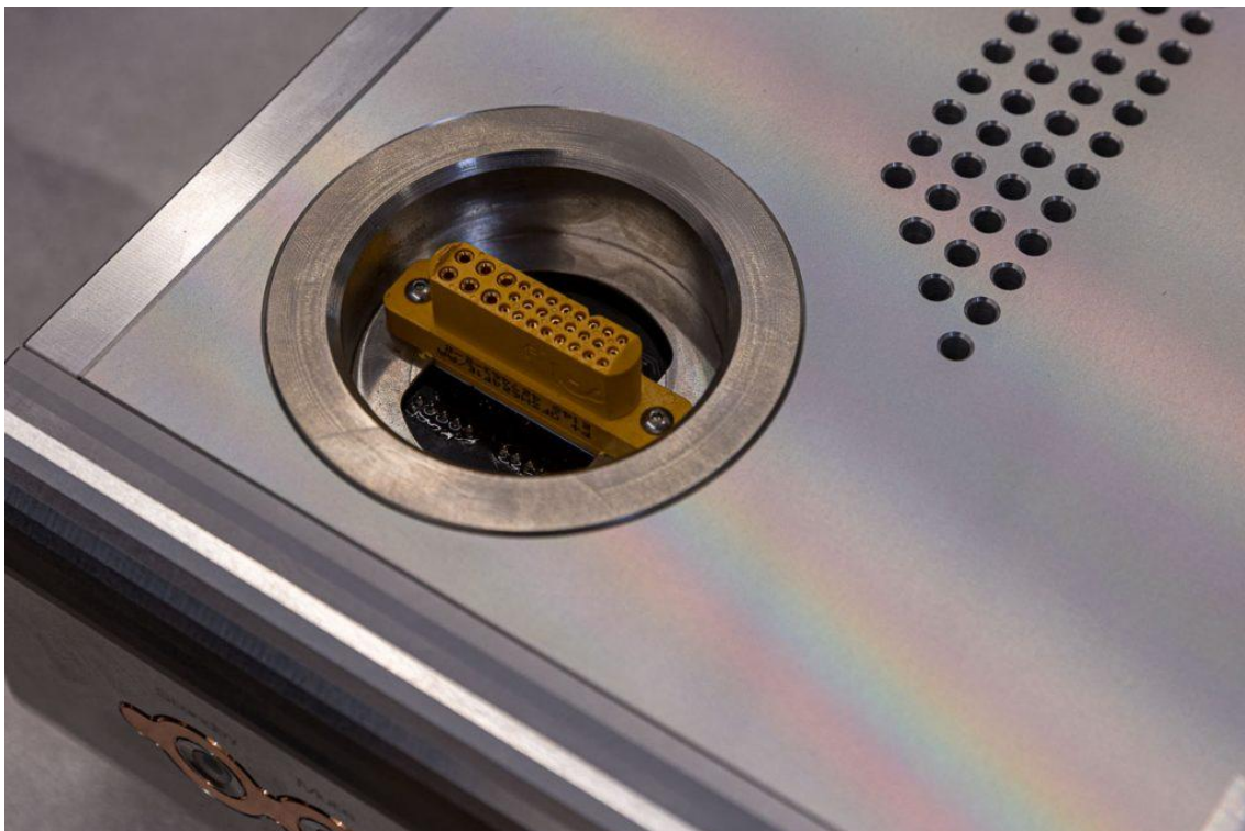
The segments of the three-piece preamp are connected via these full metal interfaces. Note the chamfered rim that makes sure that the upper piece will glide precisely into the contacts under its own weight.
