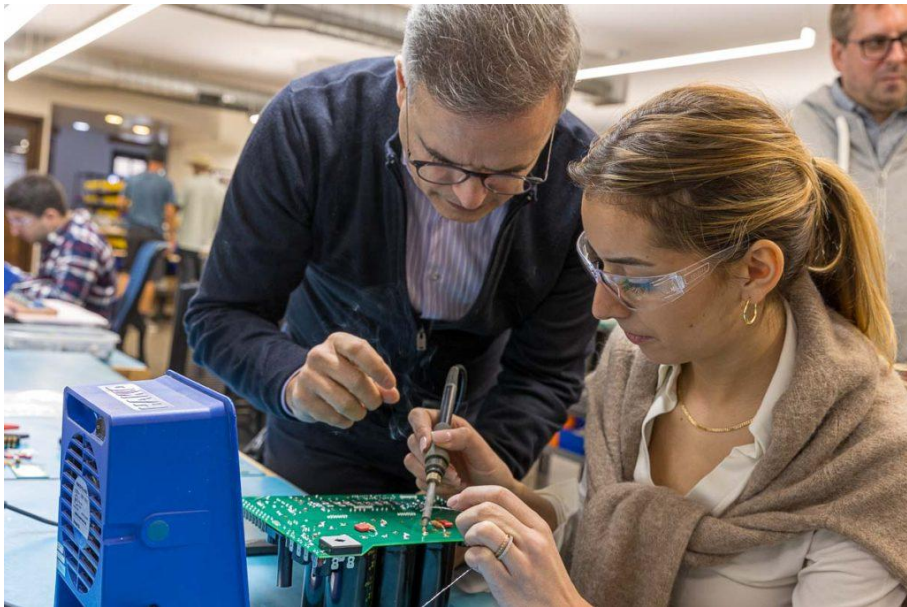
We, too, were allowed to have a go: Audio Reference CEO Mansour Mamaghani is giving his daughter Nathalie a bit of advice. The piece being worked on is the power supply for a M400 MxV power amp.
